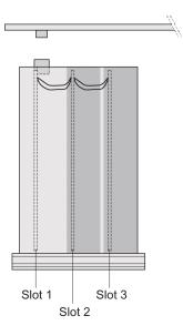
Frame type plug-in unit, non-shielded, perforated top / bottom cover, rear panel with cutout for one connector.
