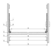
Vertical profile enables the EMC contact between the side panel and the backplane. The assembly grid is 30 mm.
