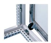
The Door Support Roller Kit supports and aligns heavy doors. Kit is suitable for all solid doors and glass window doors. Kit is not recommended for use on solid doors with door bars removed or polycarbonate window doors. Drill points in window door brackets for mounting Door Stop Kit.
