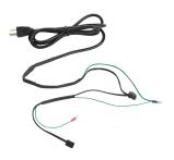
Use to power 120 VAC Compact Axial Fans; replaces existing supplied power cord. Fan cord includes inline thermostat. Fan(s) will turn on when the inline thermostat reaches 86F (30C). Fan(s) will run only when temperature is above 86F (30C). Use with 110-120 VAC fans with power cords only. One or two fans can be used with power cord.
