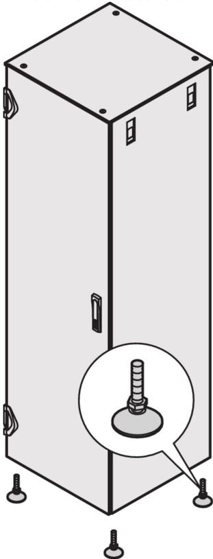
Adjustable feet or feel levellers fit into the bottom of a rack. It helps maintain rack stability in uneven surfaces and for wire shelving.
