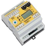
nVent RAYCHEM TraceTek TTSIM-2 is a sensor interface module with capacity to monitor up to 150m (500ft) of sensor cable. Leak alarm signaling is via 3-digit leak location on built-in LCD display, LED, dry contact relay, and serial data to a PLC or host system using standard protocols. It can be used as a stand-alone leak detection alarm unit, or in networks with other TTSIM, TT-NRM, TTDM-128, or TT-TS12 modules. Available in 24, 120 or 230 Vac 50/60 Hz or 12 or 24 Vdc.
