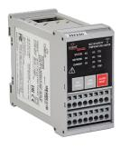
nVent RAYCHEM NGC-40 Series - Temperature Limiter Module is a safety temperature limiter module. It can be used with up to 3 temperature inputs for three phase heat-tracing circuits, with one output for the contactor and another for external alarm annunciation. The safety temperature limiter can be reset by digital input, through the user interface Touch 1500 or nVent RAYCHEM Supervisor.
