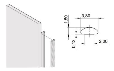
The textile EMC gaskets are inserted into a slot on the right hand side of the U-shaped front panels. The gaskets are glued to the front panel.
