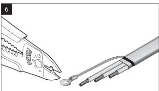
Use a Thomas and Betts WT2000 crimp tool to crimp the ring terminal onto the braid.
