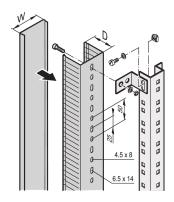
Cable ducting in side and rear cabinet areas and mounting on cabinet uprights, depth members or C-profiles.
