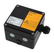
nVent RAYCHEM JB-EX-XX are junction boxes with or without earth plate and external earth stud. Depending on the type, they are equipped with 10 mm² or 35 mm² terminals to allow loads up to 100 A to a power supply or other configurations such as Tees or Splices. Available in different sizes with a various number of M20 entries to accommodate multple configurations and electrical loads.
