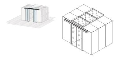
Aisle closing doors in different versions manual and automatic opening.
