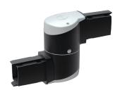
Syspend 281-Max Intermediate Joint to join two horizontal tubes together for a longer run. Arm can be rotated or turned 300 degrees. Includes safety stop and maintenance-free bearing. Use of the Intermediate Joint reduces the system load capacity to 179 lb. (81.2 kg) at 3.3 ft. (1 m).
