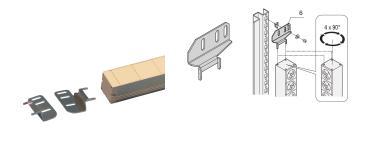
Assembly kits for PDUs. Allows easy integration of PDUs in a rack.
