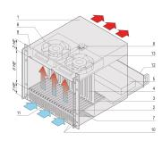
VME64 system for 21 VME64x boards 6 U, 160 mm. Rear I/O option The power for the system is supplied by a open frame power supply. A fan control module monitors the fans, the temperature and voltage.
