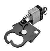
Dual-Access Safety Lockouts provide a means of using two padlocks on a secured power source. Either padlock can be removed enabling power to be interrupted and enclosure accessed. Padlock holes are .38-in. (10-mm) in diameter.
