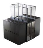
Works with a pod of cabinets surrounding a hot aisle. It is supported on top of the cabinets and channels the hot air exhausted from the server equipment housed inside the cabinets up to a ceiling plenum. This is used to completely separate the hot from cold air, drastically reducing data center energy costs.
