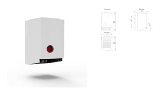
The high performance heater, ECR, with an integrated thermostat and a heating capacity of 550 watts, uses a fan to distribute the heat generated evenly throughout the enclosure, which means hot spots can be prevented. Water condensation is eliminated, also when the ambient temperature drops sharply. The preinstalled integrated thermostat will save space inside the enclosure and reduce installation time compared with a thermostat mounted separately.
