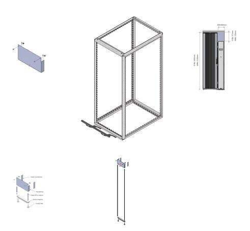
The RackChiller In-Row Ganging kit allows for integration of the cooler into Proline or Varistar aisle containments. The included levelling feet, plinth and top blanking panel assure seamless look while providing best sealing properties of the aisle containment. The kit is available in different variations, depending on the cooler and racks used.
