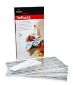
nVent RAYCHEM T2Reflecta is an underfloor heating insulation and heat spreading board used with T2Red heating cable to improve energy efficiency and optimise comfort. Suitable for renovation and new build. Available in 1  $\rm m^2$  and 3  $\rm m^2$  packs.
