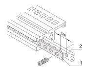
Perforated strip out of 1mm Aluminum for centering shielded plug-in units.
