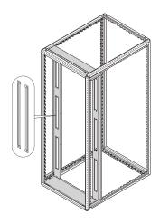
Brush strip to close 2 U by 19" cutouts for air management blanking panles. Square hole mounting with cage nuts.
