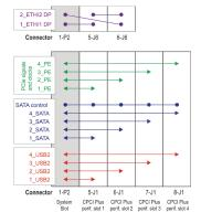
4 U CompactPCI PlusIO System with vertical Card Cage for one CPCI PlusIO System Controller, 4 CompactPCI and 3 CompactPCI Serial Peripheral Boards and one CompactPCI 3 U Pluggable Power Supply.
