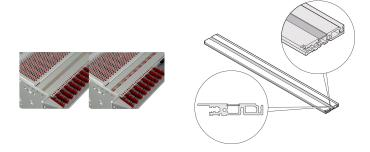
The cover strip can be inserted into a groove on the rugged horizontal rail and covers the perforation of the horizontal rail for fixing the guide rails.
