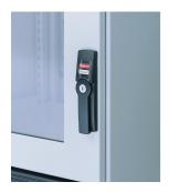
Small Flush Swing Handle is used on smaller doors less than 800mm (31.5 inch) in height that have two-point latching. Handles are ergonomically designed to provide style and function in a low profile. They can be installed to rotate either clockwise or counterclockwise. The shape of the design provides aesthetic compatibility with the Flush Swing Handles. This handle includes keylocking provision, two keys, provision to add your logo.
