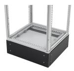
Plinth Bases install under an enclosure to provide space for cables to enter from below. A Plinth Base consists of eight corner supports connected to four access panels. The corner supports are cast aluminum. The access panels attach to the corner supports with screws. Plinth Bases include all necessary mounting hardware. Order a gland plate system to provide Type 12 protection when using a plinth base.
