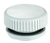
Pressure differentials in a tightly sealed enclosure result from heat generated by electrical and electronic equipment within the enclosure and fluctuations of outside ambient temperature. Pressure compensation devices provide IP66 protection in applications requiring slow pressure equalization. For optimal performance, install two plugs diagonally to each other.
