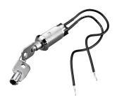
Enables authorized personnel to enter an enclosure while the enclosure contents are energized. Defeater is a key-operated momentary contact switch with contacts normally closed. Turning the key disengages the circuit to the electrical interlock.
