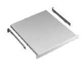
The Rack-Mount Adjustable Shelf mounts to the front surface of front and back rack angles. The adjustable shelf support brackets are clear-plated 12 gauge steel and adjustable to fit multiple-depth enclosures or rack angle placement. There are both solid and vented models available. They fit 19- or 23-inch rack spacing and require only 1U of rack space. Please note the load rating is for 150 lb. (68 kg).
