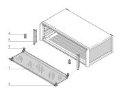
The front hood bottom hinged can be assembled on to a PropacPRO case. It protects the PCB from accidental operations. A retrofittable lock can be installed.
