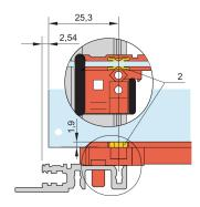
New generation of accessory type guide rails for PCBs or plug-in units. Forms a reliable interface between the subrack mechanics and the sub-assemblies.
