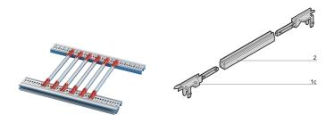
Plastic end pieces for individual multi-piece guide rails with plastic or extrusion mid-piece. Available as Standard, Acessory or 4.4" PCB types. End pieces can be optional equipped with a ESD clip, which ensures conductive contact between PCB and horizontal rail. Suitable for RatiopacPRO/-AIR, PropacPRO, CompacPRO and EuropacPRO.
