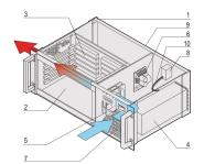
VME system for 5 horizontally mounted VME boards 6 U, 160 mm. The power for the system is supplied by an open frame power supply. A fan control module monitors the fans, the temperature and voltage.
