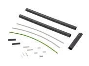
nVent RAYCHEM CS20-2.5-PI-NH is a heat shrinkable polymer kit for the connection and termination of polymer insulated (PI) series resistance heating cables to cold leads. The kit is designed for use with junction boxes with M20 entries and allows to terminate circuits up to 25 A. The kit includes all materials for heating cable and cold lead connection, as well as the glands to terminate the cold lead in the junction box.
