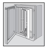
Swing Frame provides 19-inch rack-mounting capabilities with U-Style (Type RA) mounting hole pattern. Quarter-turn latch has 100-degree swing. Adjustable mounting provision. Swing frame maintains enclosure rating if properly installed in an nVent HOFFMAN enclosure. Front mounting position is approximately 140mm (5.5 inch) back on 400mm enclosures. Includes mounting hardware and instruction manual.
