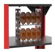
The coil storage rack helps organize cable and wire spools to improve the safety and efficiency of the cable management system and increase the Personal Wiring Assistant (PWA) machine performance. Each rack can accommodate up to eight coils, each with a maximum 200 mm flange diameter x 85 mm width.
