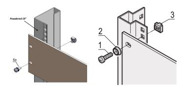
For standard grounding use a grounding nut and washer on at least one attachment point.
