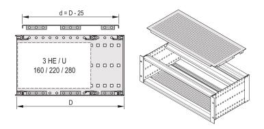
A cover plate is used for electromagnetic shielding or as mechanical protection. The cover can be screwed onto the side panel.
