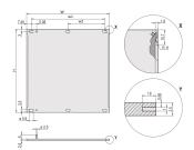
Flat front panel. Shieldable with stainless steel EMC gasket.
