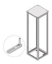
Tip-Over Protection helps make floor mounted enclosures stable and prevents tip overs due to load imballance. The tip over protector can be assembled on the frame or the plinth.
