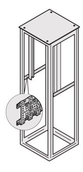
Horizontal depth member in the cabinet depth. Mounted directly at the Varistar CP frame for cable management, increased frame stiffness and additional fixing points.
