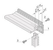
Z-rail for connector in accordance with EN 60603-2 (DIN 41612).
