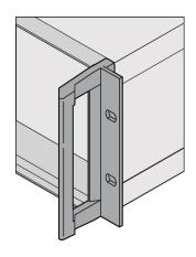
With this 19" mounting bracket with handles the flexible and robust RatiopacPRO/-AIR case, is simple to convert from desktop to 19" rack-mountable.
