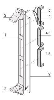
U-shaped front panel with cutout for PMC. Shieldable for textile EMC gasket.
