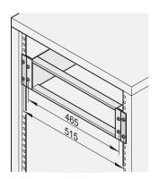
The 19" adaptor allows 19" components to be installed in the metric Etsirack.
