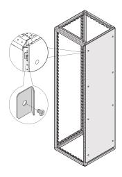
The internal retainer is easily fitted without drilling, and allows the side panel to be removed only from inside. The retainer is only for IP 20 applications.
