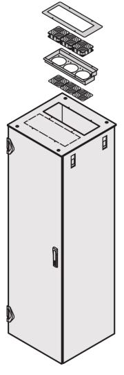
Fan Tray allows easy active cooling through fans with IEC320 connection. The Varistar fan tray is ideal for flat top covers with cut out zones.
