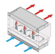
Air deflector with 1 U height to guide the air from front to top or from bottom to rear.
