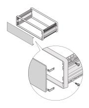
The front panel for CompacPRO Case mounts to the frame of the case. The front panel has no visible screws and can be used for front foil.
