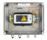
The nVent RAYCHEM ACS-30-EU-ELEXANT650C-SMDI-MOD Module for the ACS-30 system provides smart sensor input for surface snow melting and roof & gutter de-icing applications. The Remote Monitoring Module (RMM) is used to collect sensor/temperature inputs for monitoring of the heat tracing circuits of an ACS-30 control system.
